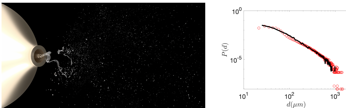
Figure 1: Left: snapshot of the liquid-gas interface in a simulation of airblast atomization. Right: comparison between droplet size distribution from simulation (line) and experiments (symbols).
