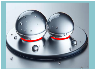
Three-phase contact line
