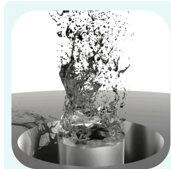
Complex liquid-gas interface close to the nozzle of a coaxial atomizer
