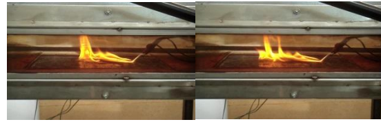
Figure 15: Fire spreading in Hidden Fire Apparatus
