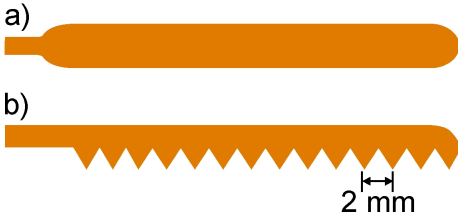
Figure 5: Top view of a smooth and serrated active electrode used in the DBD plasma actuators
